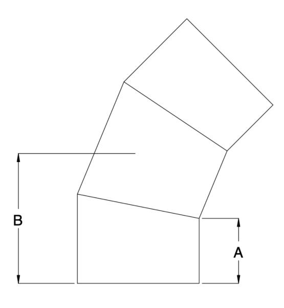
Fittings between 20" and 48" are designed to be fused on a 1648 or smaller field machine, If longer lengths are required, please contact Sandale Utility Products for special requirements.
