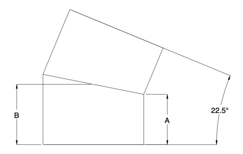
Fittings between 20" and 48" are designed to be fused on a 1648 or smaller field machine, If longer lengths are required, please contact Sandale Utility Products for special requirements.
